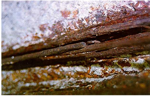
Figure 4-7 Broken wires of a corroded tendon
