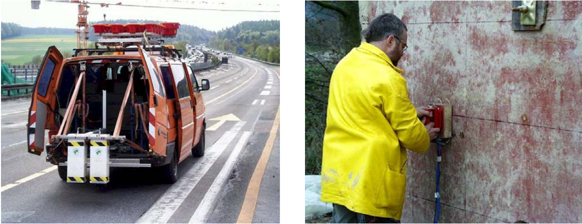
Figure 5-3 Undertaking GPR surveys
