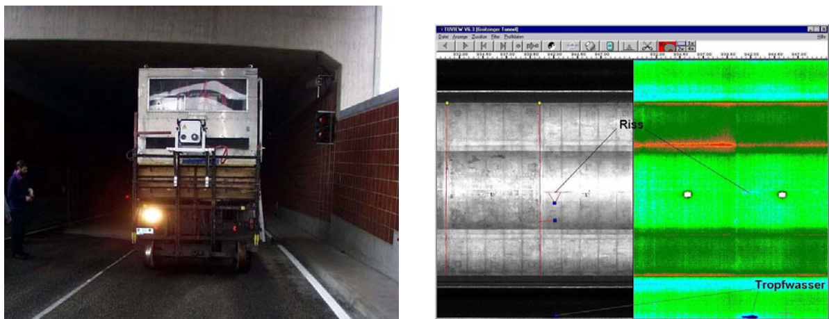
Figure 5-9 The use of a laser scanner in a tunnel, and an example of the output
