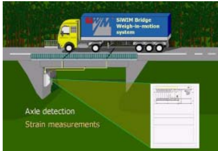
Figure D.6: Bridge WIM instrumentation
